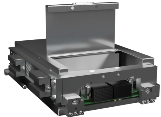
ML7064E-LX 64 channel 112 Gbps/lane BERT for 128 differential pairs/unit
